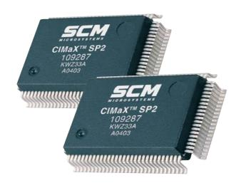
Dual slot CableCARD™, DVB Common Interface and OpenCable™ hardware controller for Digital TV receivers
